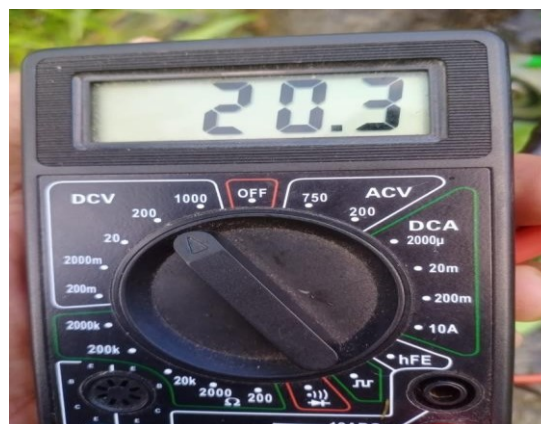
Figure 6. Generator Voltage Measurement for 3 Minutes
