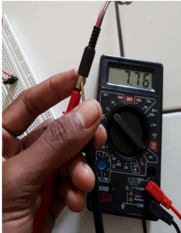
Figure 6. HC-05 Bluetooth Voltage Measurement
