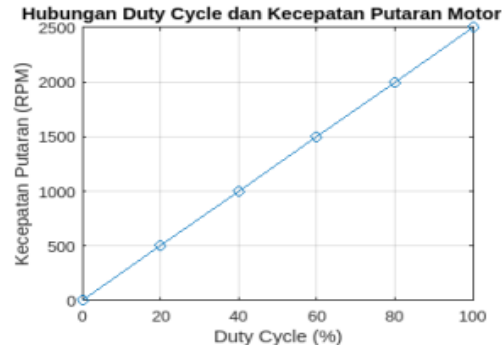
Figure 3. Graph of the correlation between duty cycle and DC motor speed
